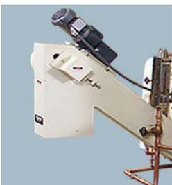
An accurate glass-tube flow meter is used to provide a fine degree of control and repeatability. This system removes virtually all grit down to 10 mesh in size and some portion of finer grit down to 40 mesh. Slurry concentrations up to 18% are achievable. Operation is simple and efficient with very low maintenance.
